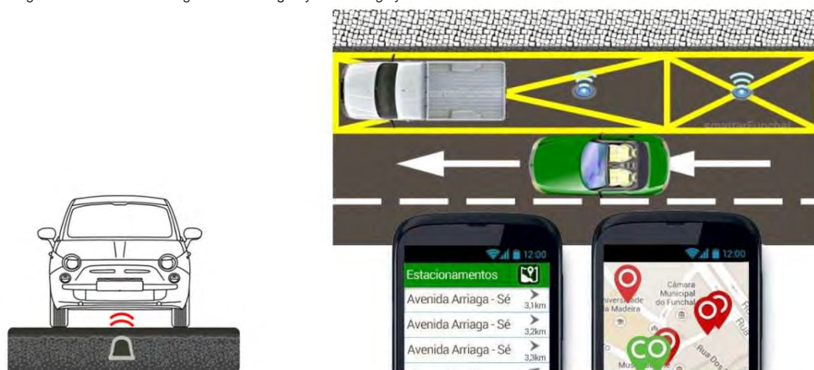
Figure 4.60 - How a loading and unloading bay monitoring system works
