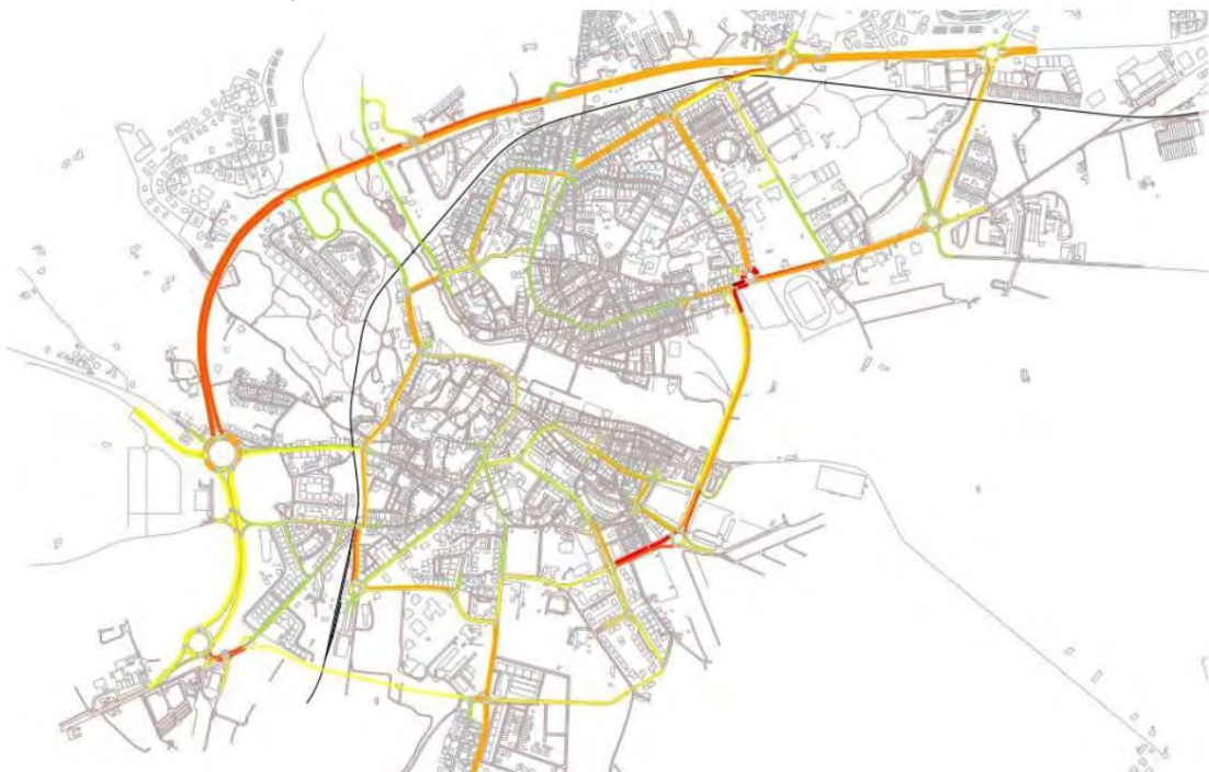
Figure 4.8 - Future road network with current traffic - PPM
