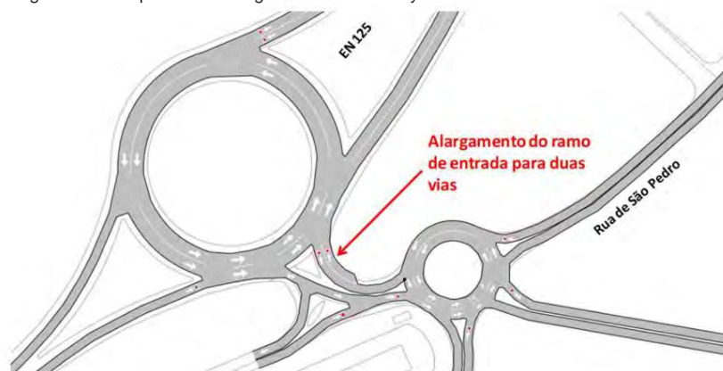
Figure 4.7 - Proposed widening of the EN125 entry branch
